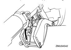
To lower the outboard motor to the normal running position, first slightly tilt the outboard motor up. Then pull up the tilt support bar lever and slowly tilt the engine down.
